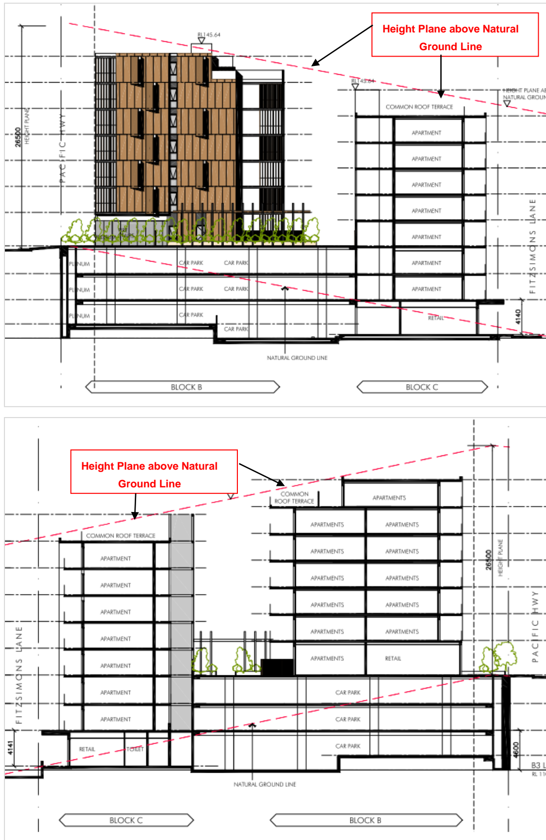
Figure 4: Cross sectional elevations of Building B and C from Pacific Highway to Fitzsimons Lane
