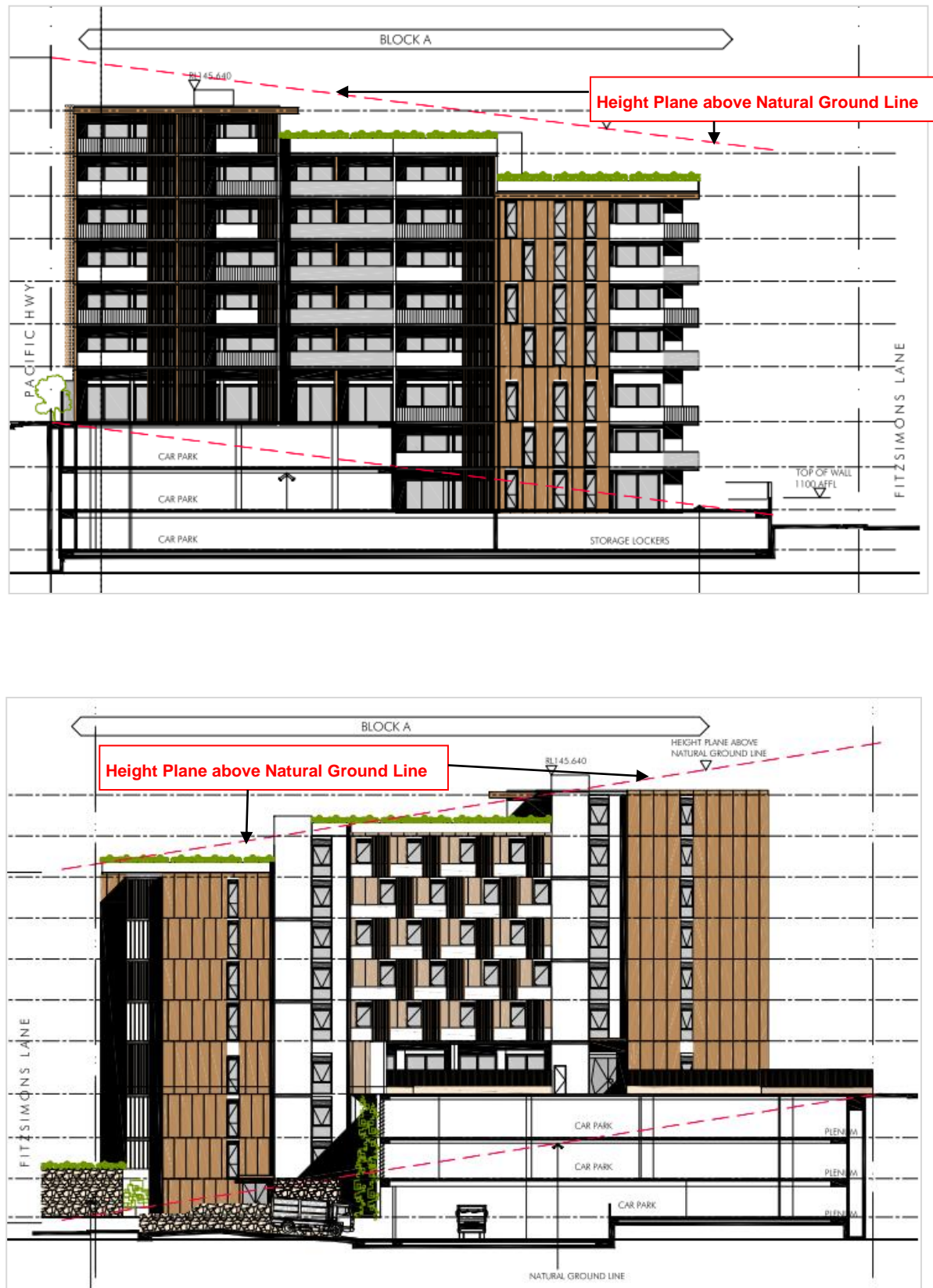
Figure 3: Cross sectional elevations of Building A from Pacific Highway to Fitzsimons Lane.
